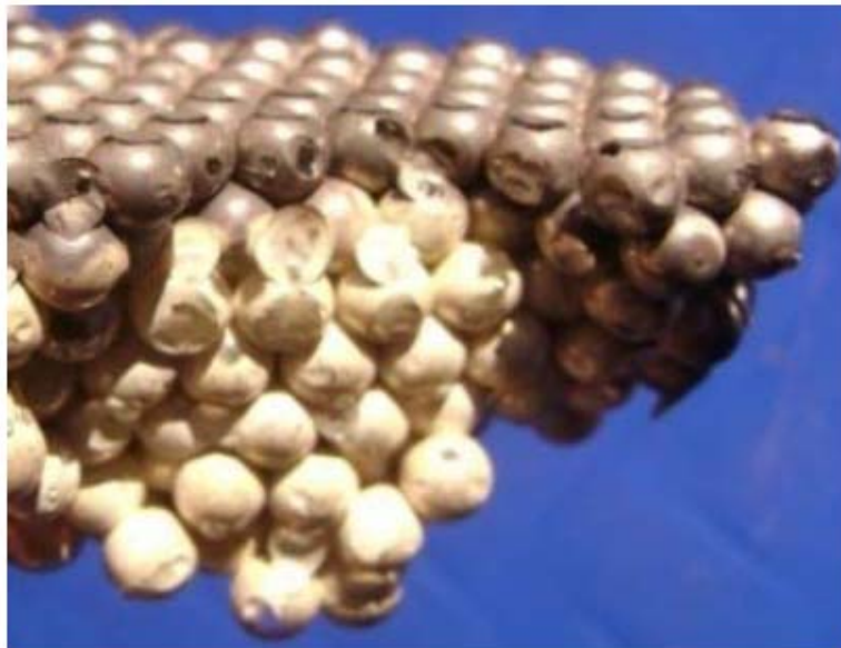
Figure 5. Yellow spheres in the inner part of opal-like glass structures coated with Ag/S/Ni.
