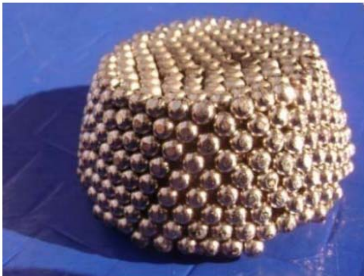
Figure 4. A glass/nickel opal-like structure.
